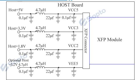
**Recommended High-speed Interface Circuit**
