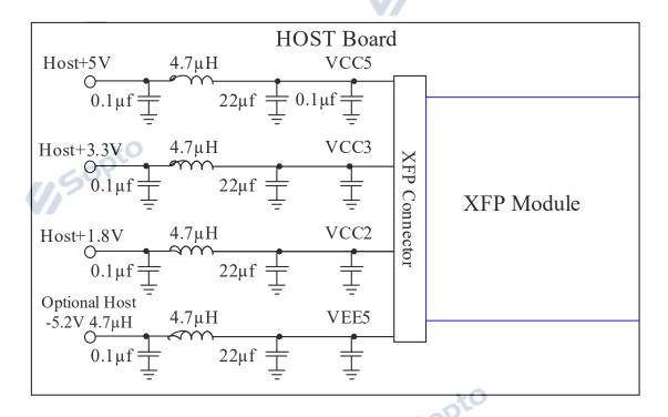
**Recommended High-speed Interface Circuit**
