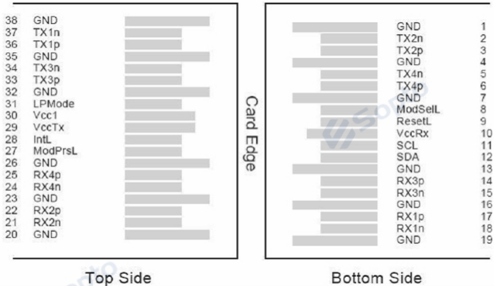
Diagram of Host Board Connector Block Pin Numbers and Name
