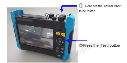
As an ideal tester of ODN and FTTx, OTDR is provided a unique built-in PON network test function, can penetrate an optical splitter of up to 1:128, and can be used to test each branch of the PON network accurately.
